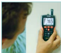
Measure moisture of wall material with non-invasive Pinless technology
