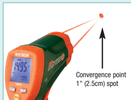
Two laser points converge at a distance of 30"/76.2cm (model 42512) and form a 1" (2.5cm) spot.
